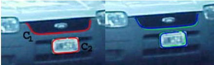
Fig. 9. Green curves in frame 2 are modeled similarity transformations of the red curves in frame 1 while blue curves are the actual curves in frame 2
