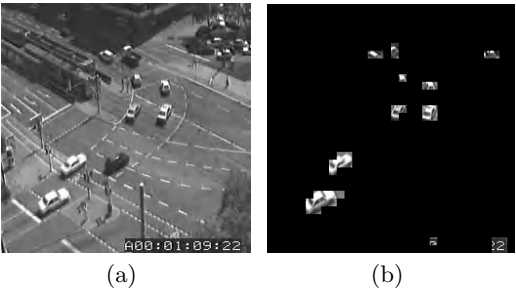
Fig. 4. \epsilon = 1 , \alpha = 0.4 , \beta = 10 , (a) original image, (b) motion detection with J=3
